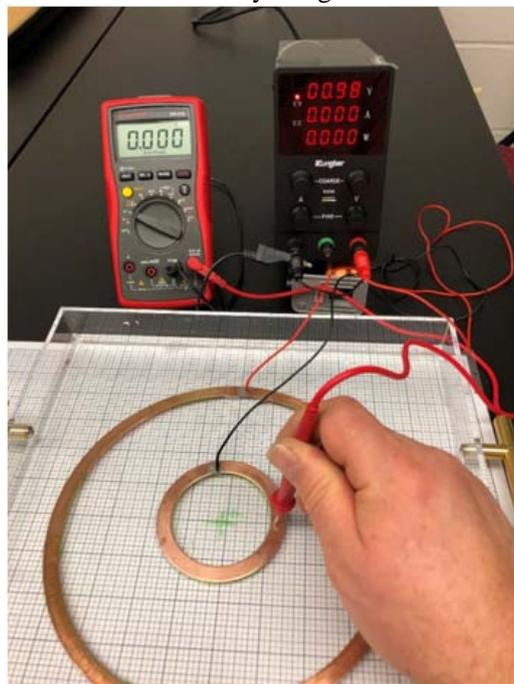
Figure 2. E-Field mapping Apparatus with tap water in a plastic tray (2022).
