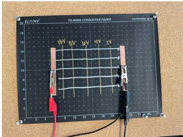
Figure 3. The Ultimate E-Field Mapping Apparatus (2022A).
