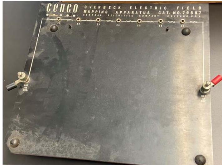
Figure 1. Overbeck's Electric Field Mapping Apparatus (1948).
